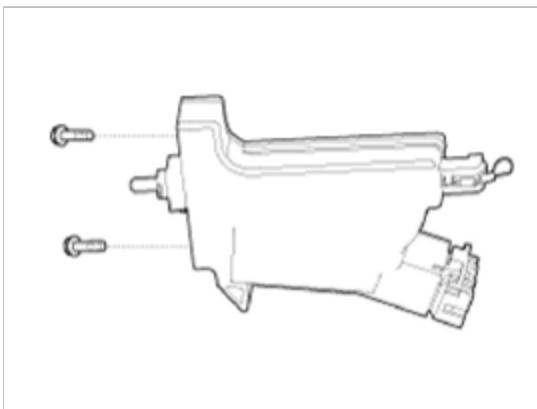
4. Check for continuity between terminal No.1 and No.2. If there is no continuity replace the fuel filler door opener.
